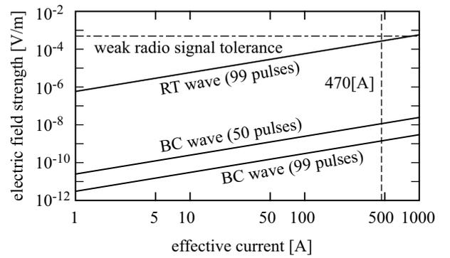
Fig. 3. Noise intensity of pulse trains at 40[kHz].
