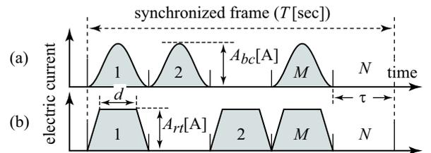
Fig. 1. Pulse trains adopted for noise spectrum evaluation.
