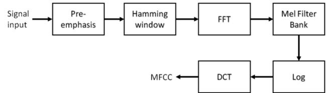
Fig. 1 MFCC block diagram
