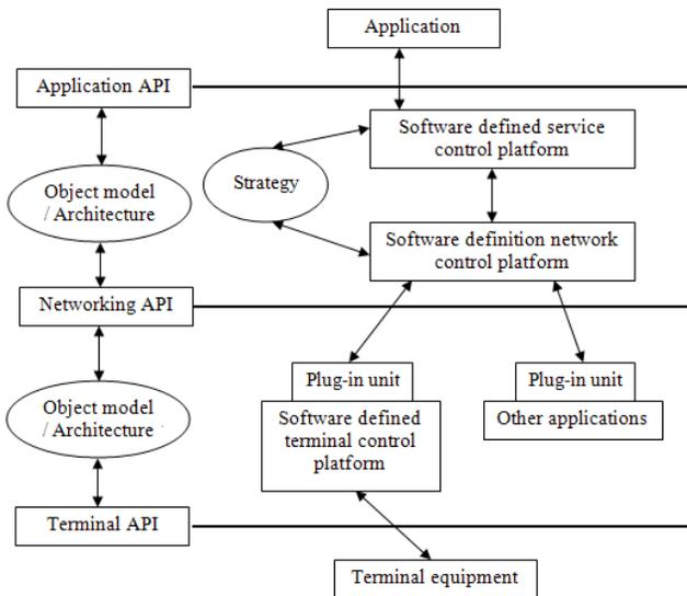
Figure 2 The architecture of the 3S platform
