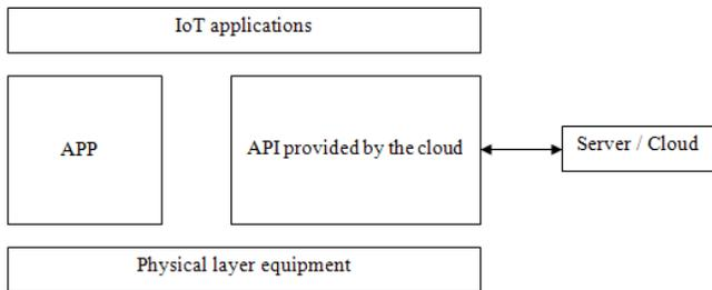
Figure 1 The architecture of the cloud-based IoT platform
