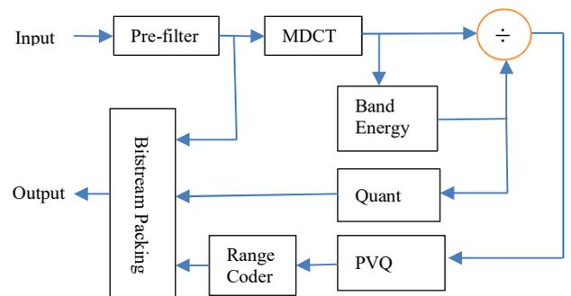
Fig. 1. Signal processing flow of the CELT coder.
