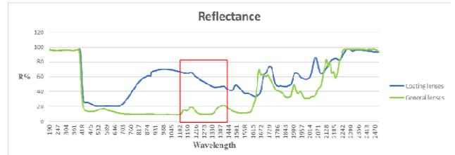
Fig. 4. Ordinary lenses and coated lenses Reflectance Relationship
