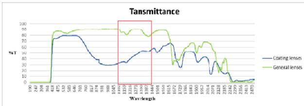
Fig. 2. Ordinary lenses and coated lenses Transmittance Relationship
