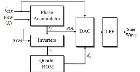
Fig. 1. Structure of a quarter-ROM DDS.
