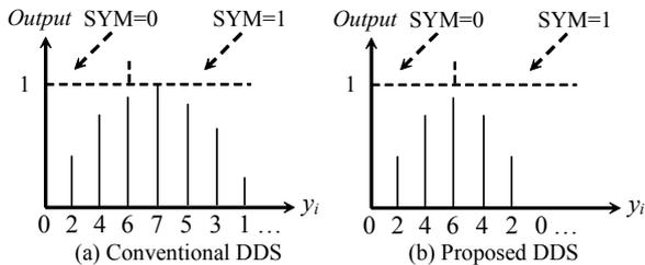
Fig. 3. Symmetry analysis for two quarter-ROM DDSs
