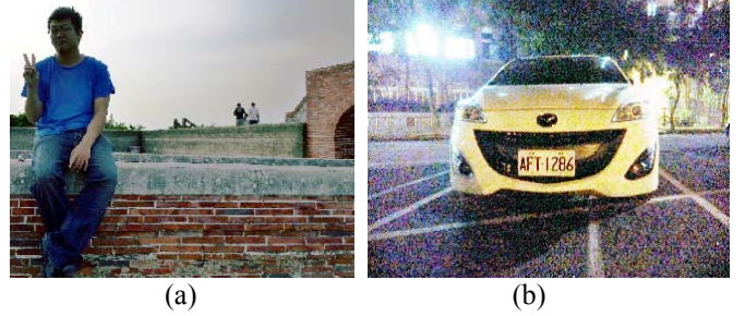
Fig.2 Enhanced results using histogram equalization. (a) Enhanced backlighting image. (b) Enhanced nighttime image.
