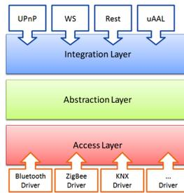
**Fig. 2.** universAAL Device discovery and integration structure
