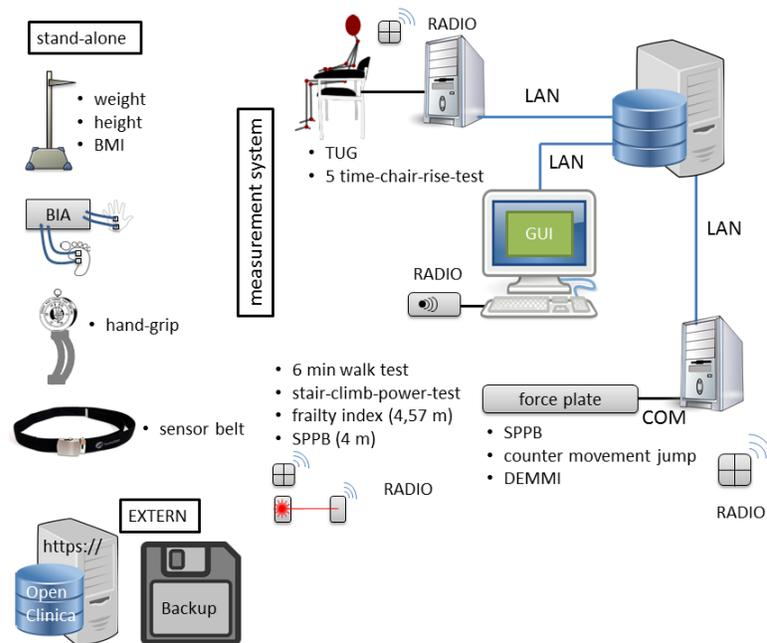
**Fig. 2** Measurement system of the technologically supported functional assessment with its single components and the corresponding assessment items, data storage and documentation.
