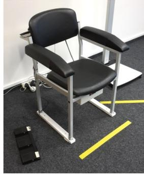
**Fig. 3** The ambient Timed Up & Go (aTUG) device includes light barriers, force sensors and a laser range scanner. The device is able to detect the sit to stand cycle and to make detailed gait analyzes.
