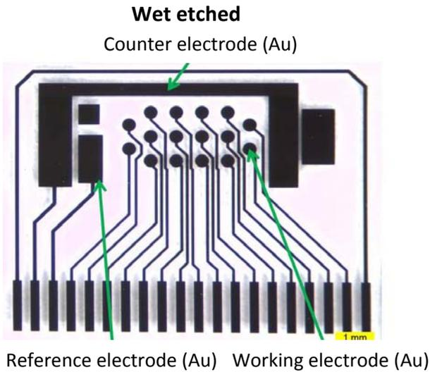
**Figure 2a** Microscopy of wet etched sensors.
