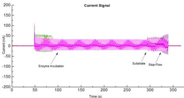
**Figure 4:** Typical current signal reading of a silicon biochip in an immunoassay, starting with incubation of the enzyme and followed by addition of substrate before stopping the flow for a reading. The different colors represent different working electrodes.
