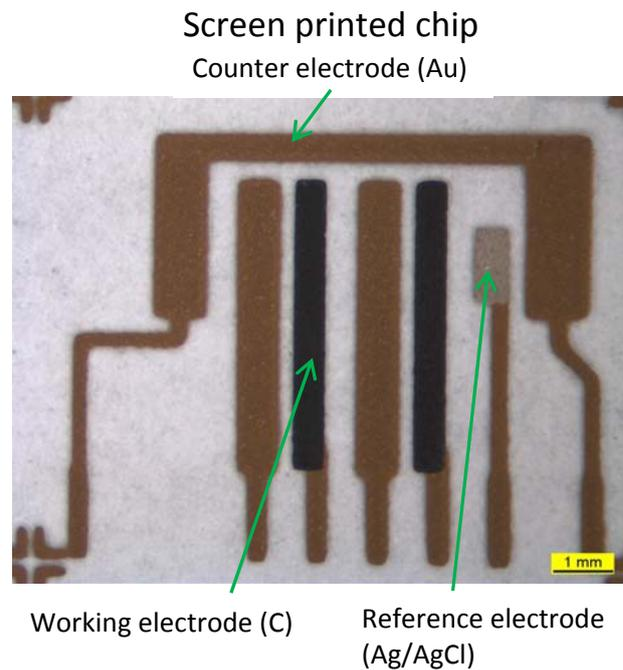
**Figure 4c** Microscopy of screen printed sensors with carbon, gold and silver-/silver chloride electrodes.
