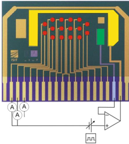
**Figure 3b:** Schematic of a multichannel potentiostat with corresponding electrode colors overlaid onto the biochip.
