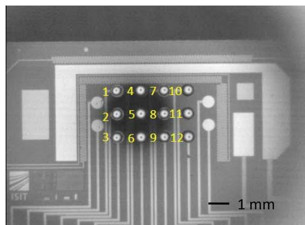
**Figure 1** Microscopy of a silicon based bio sensor.
