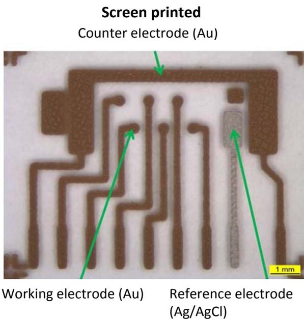
**Figure 3b** Microscopy of screen printed (no dielectric) sensors.
