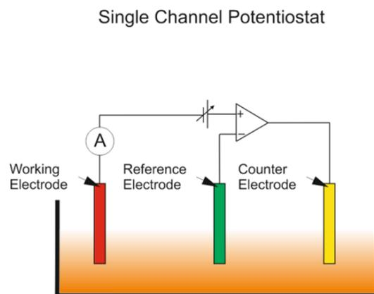
**Figure 3a:** Schematic of a single channel potentiostat
