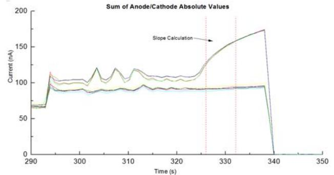
**Figure 5:** Sum of the absolute values of anode and cathode readings during the substrate and stop-flow phases. Slope values are calculated using linear regression within the dotted lines.
