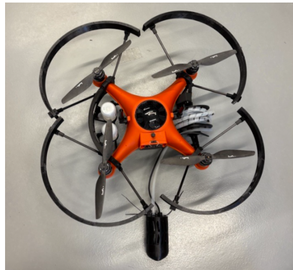
Fig. 1. Full drone system with propeller guards, water sampling mechanism, and sensor implementation on a SwellPro Fd3 Fishing Drone.
