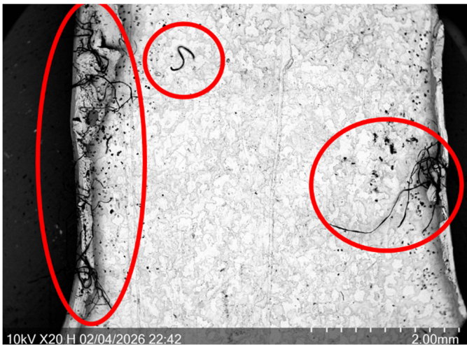
Fig. 4. Zinc whiskers observed in the curve region of the sample with 1.905 mm of elongation
