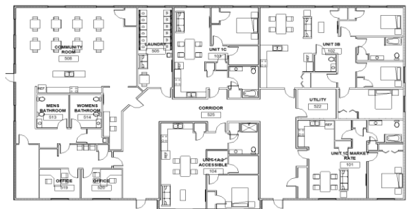
Fig. 1. Sample architectural floor plan used as the basis for MEP space generation. The layout illustrates room boundaries, spatial organization, and functional zones that are extracted from the linked architectural model and used to automate MEP space placement and parameter mapping within the Revit environment.
