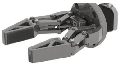
Fig. 4. CAD rendering of an open source two-finger servo motor gripper [16]. This shows the bilateral pivoted mounted PLA finger arms with triangular lightening cut-outs; the symmetric four bar linkage that connects the servo horn to each finger; and the cylindrical servo motor mounting position located at the back of the assembly.
