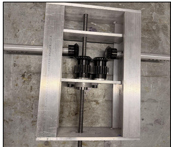
Fig. 3: Prototype of the center housing for the miter gears and spur gears connected to the ACM lead screw.
