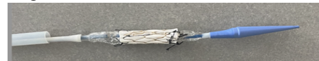
Figure 7. Prototype: Collapsed NuMed CP Stent & 0.5-mm ePTFE Conduit Crimped on Ensemble II Delivery System.
