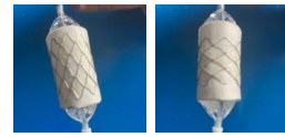
Figure 5. Expanded NuMed CP Stent and 1-mm ePTFE Conduit (Left) and Warped NuMed CP Stent and 1-mm ePTFE Conduit. (Right)
