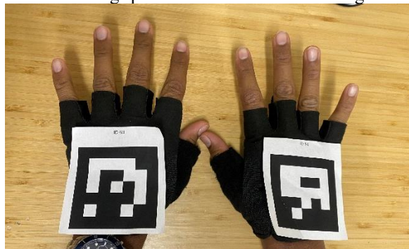
Fig. 3: ArUco Markers on gloves to track grip width
