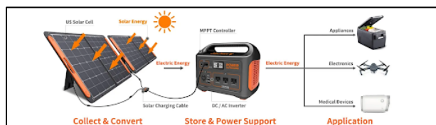
Figure 2. Schematic of a solar generator system
