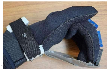
Figure 1. Side view of CAE (resistance bands are held in place by bending around the fingertip, and secured at the wrist with a screwed down plate)
