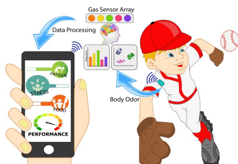
Fig 1. The concept of gas sensor arrays with sports applications for the athlete's performance and health status monitoring.
