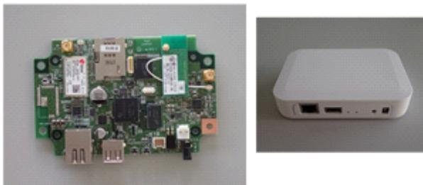
Fig. 3. Digital Grid Controller
