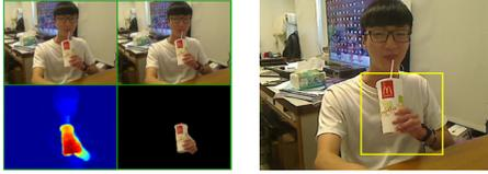
**Fig. 2.** Foreground segmentation using optical flow and Object region cropped around the object centroid
