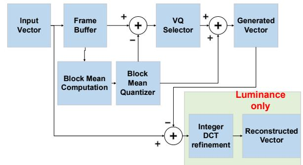
Fig. 3. Vector quantization and the residual refinement scheme
