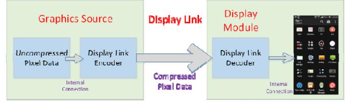
Fig. 1. Embedded image compression codec for display link
