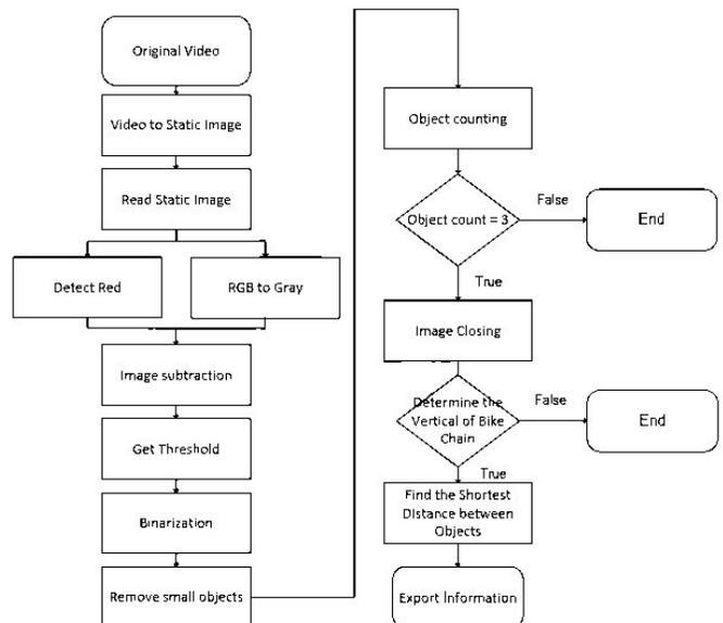
Fig. 2. The identification algorithm of bicycle objects.
