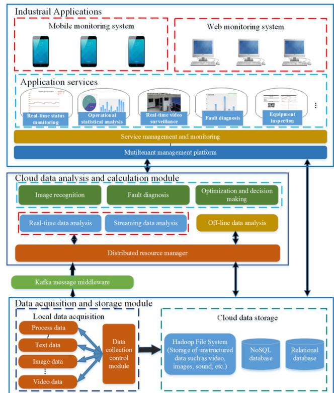
Fig. 1. Monitoring platform architecture for mineral processing equipment.
