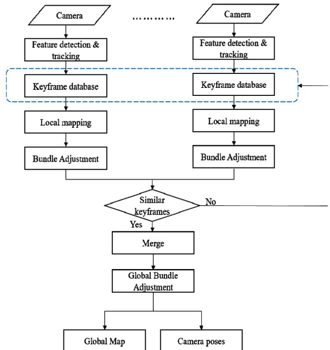
Fig. 1. Flowchart of cooperative SLAM algorithm.
