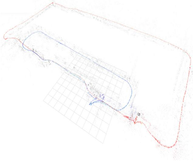
Fig. 2. Merged SLAM map of two cameras.
