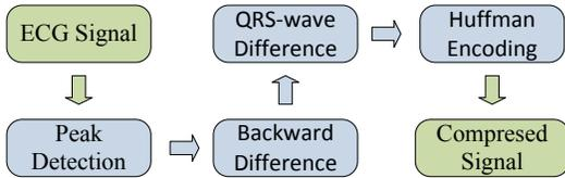
Fig. 3. Flowchart of the proposed lossless ECG compression.
