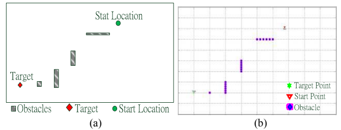
Fig. 2. Map model generation: (a) Real area floorplan (b) Map model.
