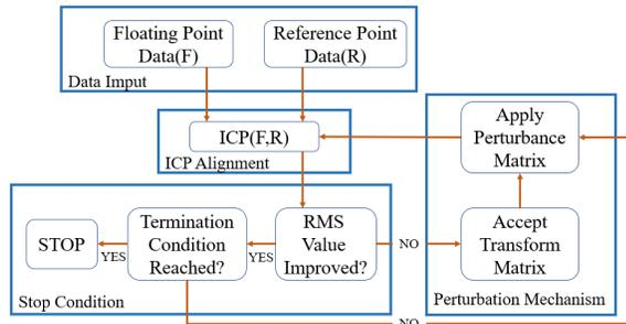
Fig 2: Flowchart of Improved Alignment (IA) Algorithm
