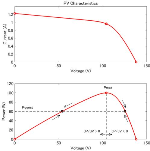
Fig. 3. Voltage-current and voltage-power characteristics of PV
