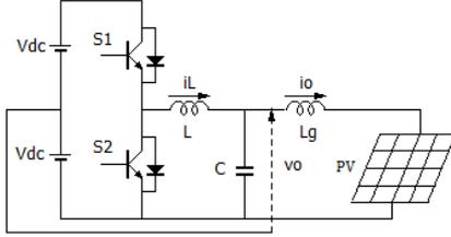
Fig. 2. PV connected inverter circuit.
