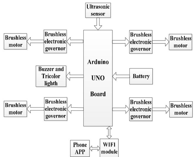
Fig. 1 The control system structure of the aircraft
