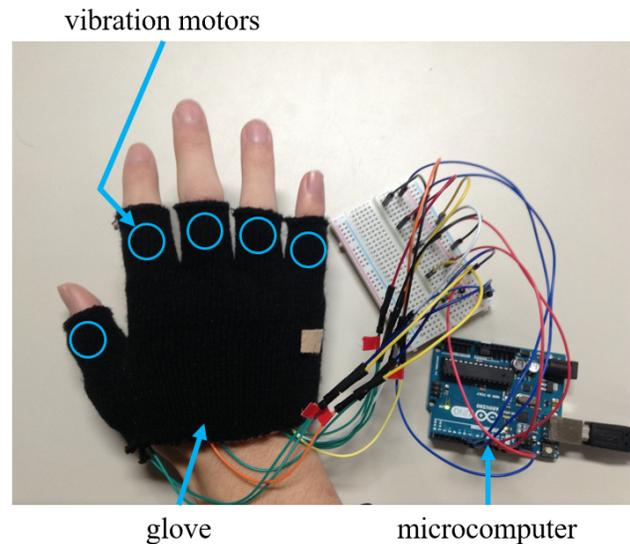
Figure 1. Handmade tactile display.
