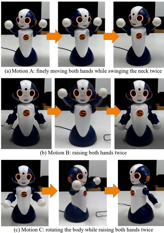
Figure 2. Robot motions used in the experiment.
