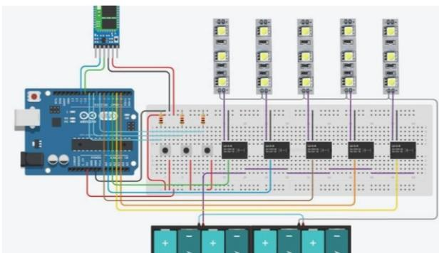
Fig. 5. The app controls several sets of LED. The separated relay and switch made it easier to manage.
