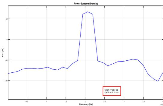
Fig 10. Frequency response of the power spectrum in the output of the 2<sup>nd</sup> order  $\Sigma\Delta$  converter with the expected 18-bit accuracy.
