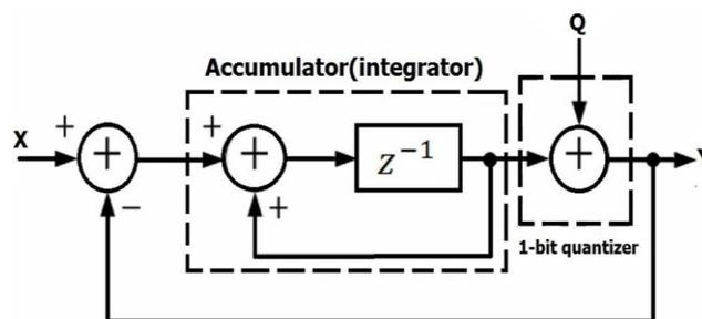
Fig 4. Block diagram of 1<sup>st</sup>  $\Sigma\Delta$  modulator.
