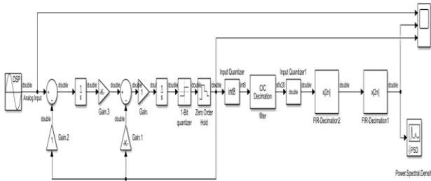
Fig7. The Sigma Delta A/D model.
