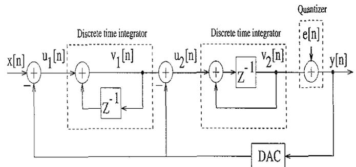
Fig. 6. Block diagram of 2<sup>nd</sup>  $\Sigma\Delta$  modulator.
