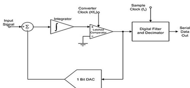
Fig3. Block diagram of A/D system  $\Sigma\Delta$ .
