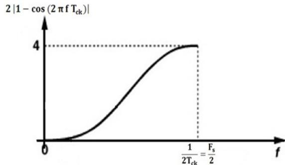
Fig. 5. Noise Shaping in the sigma-delta first order.
