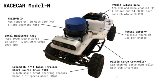
Figure 1. RACECAR-N with most important components highlighted.
