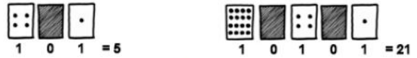
The left example is 101. That equals the decimal number 5. The right example is 10101. That equals the decimal number 21.
