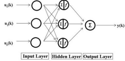
Fig. 1. NN structure used in this work
