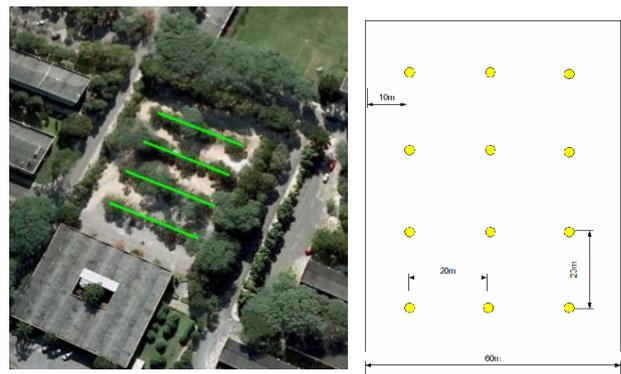
Fig 7 – Local of installation of new pole lightings (A) new pole lighting distribution (B)
