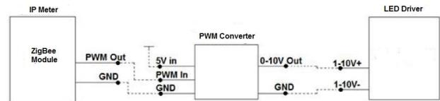
Fig 4 – Diagram connection between street light meter and LED luminaire driver.
