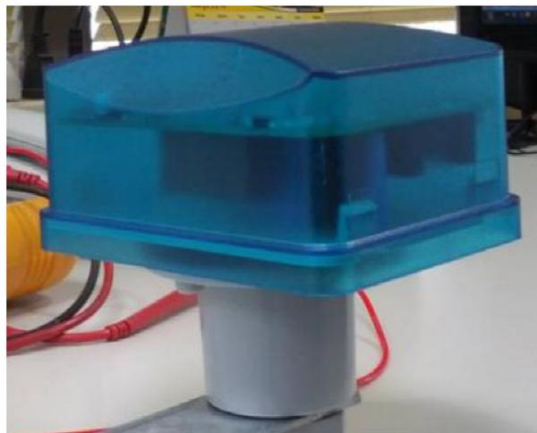
Fig 1 – Street Light Meter connected on the standard base of the conventional photoelectric sensor.
