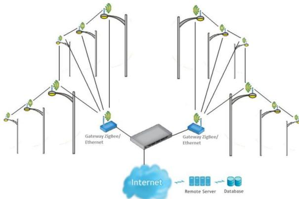
Fig 3 – Mesh network architecture for street light meters.
