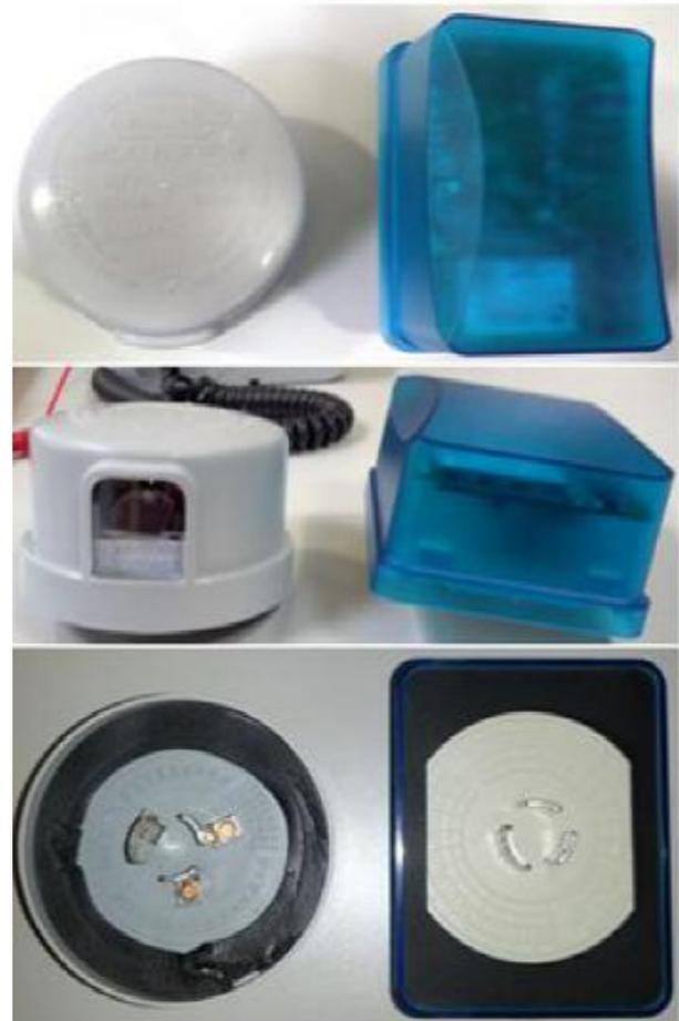
Fig 5 – Street light meter with final product compared with the conventional photoelectric sensor.
