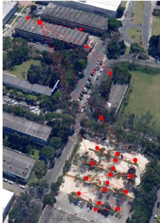
Fig 10 – Position of each measuring device and the routing routes for communication with an internet gateway
