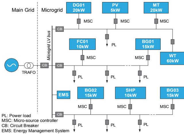
Figure 2. Microgrid conceptual scheme. Based on [22].
