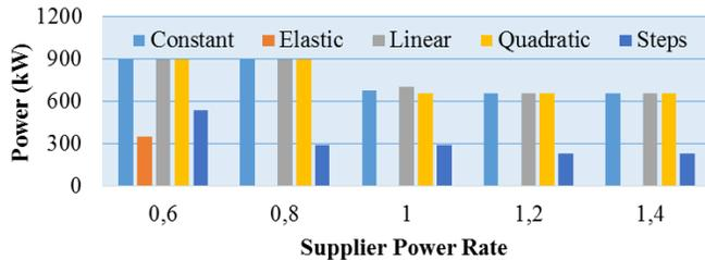
Figure 2 – Consumption reduction by DR program and supplier power rate.
