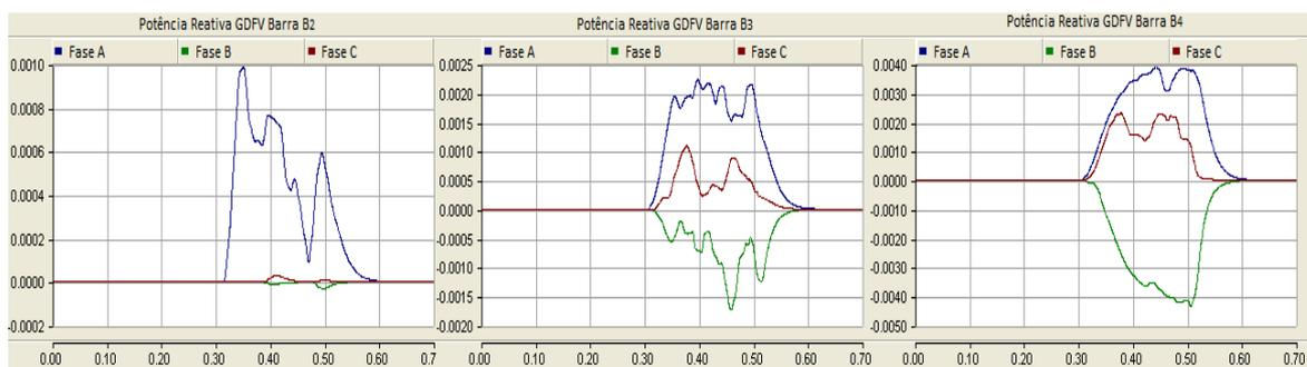
(b) Three Phase Reactive Power Injection/Absorption
