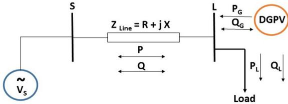
Fig. 1. Two-Node Equivalent Distribution System with DGPV Source
