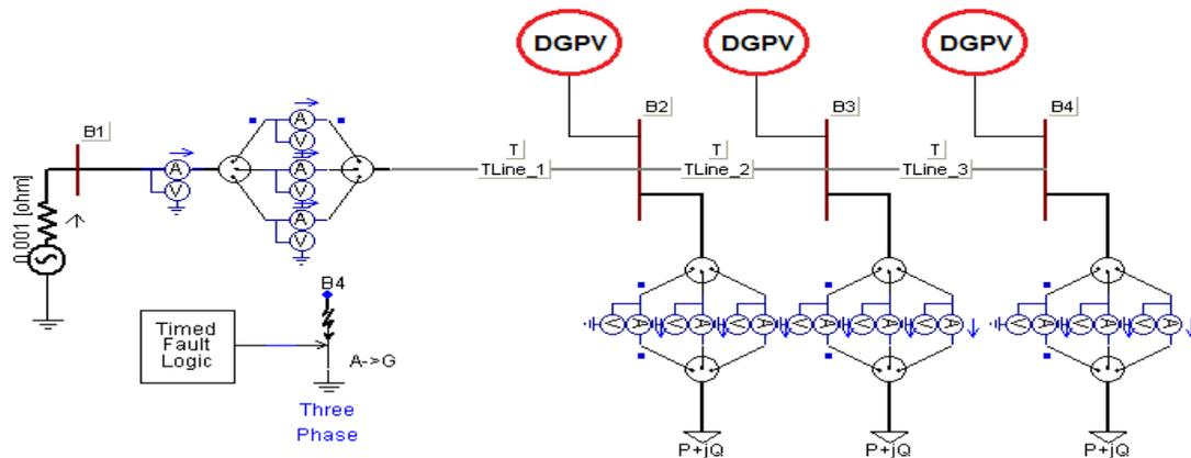
Fig. 5. Distribution Network Modeling for Voltage Regulation Support Simulations
