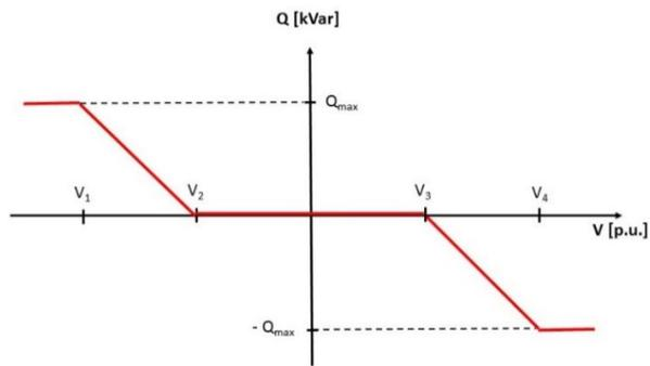
Fig. 4.  $Q(U)$  Method – Characteristic Curve
