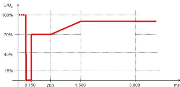
Fig. 2. Fault Ride Through Capability – Germany Grid code [8]
