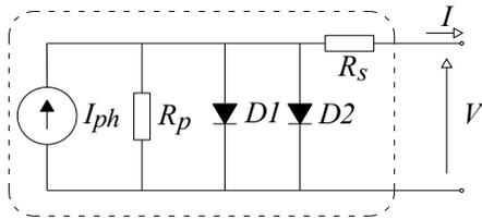
Figure 1. Equivalent electrical circuit of a polycrystalline solar cell: the “double diode model”.
