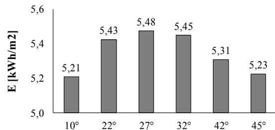
Figure 2. Average annual irradiation effectively collected by a  $1 \text{ m}^2$  PV panel placed at different orientation angles (in Santa Fe, with azimuth  $= 0^\circ$ ).
