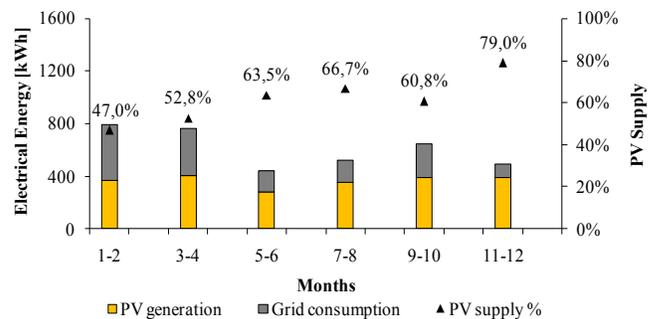
Figure 5. Energy balance for a residential user with an installed PV system of 1,290 W. (Triangles indicate the bimonthly fraction of the electric energy that could be covered with PV generation)
