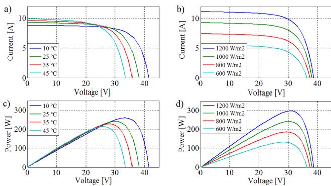
Figure 3. Characteristic curves for a polycrystalline panel of 240 Wp according to the PV model at: (a, c)  $E = 1,000$  W/m<sup>2</sup> and different ambient temperatures; (b, d)  $T = 25$  °C and different irradiances levels.
