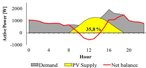
Figure 4. Comparison of required and produced instantaneous active powers for a typical dwelling when using a PV system of 1,290 W (results corresponding to January, 22<sup>nd</sup>). The red curve represents the net balance.
