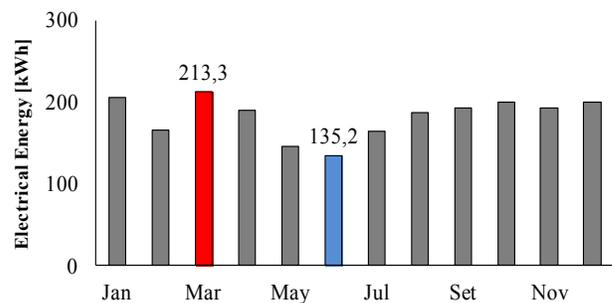
Figure 6. Electric energy that could be generated with a residential PV system of 1,290 W.
