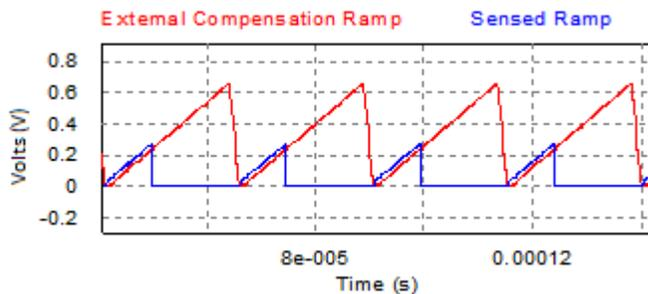
Figure 5. Sensed ramp  $S_n$  and external compensation ramp  $S_e$ .
