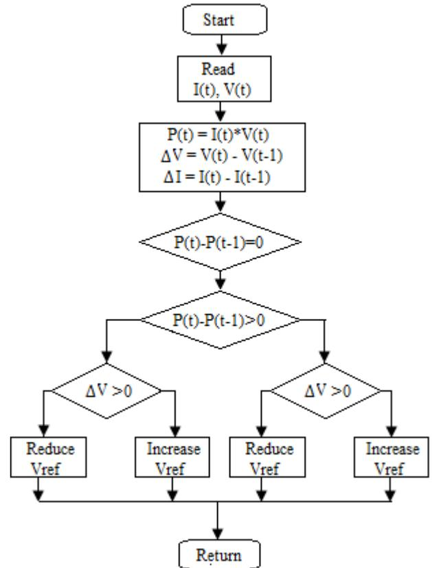
Figure 4. Flowchart of P&amp;O algorithm.
