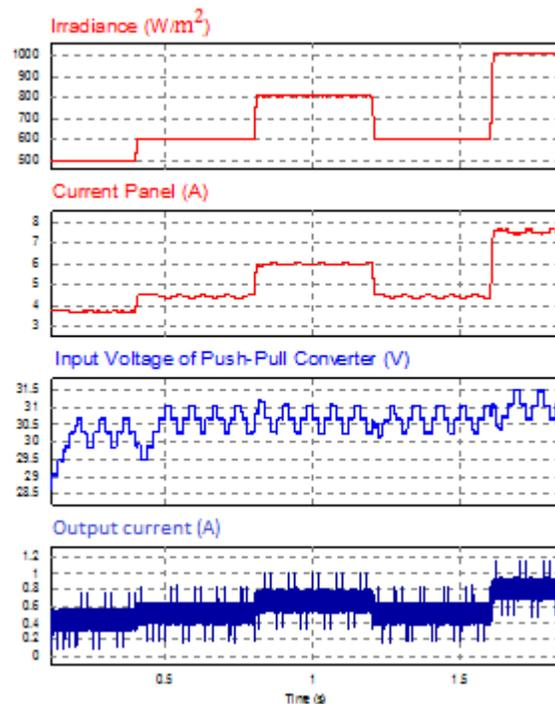
Figure 8. Main waveforms of voltage and current of the push-pull according to changes of irradiance.
