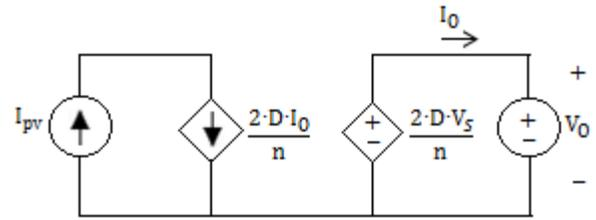
Figure 1. Equivalent circuit of the push-pull at the operating point.
