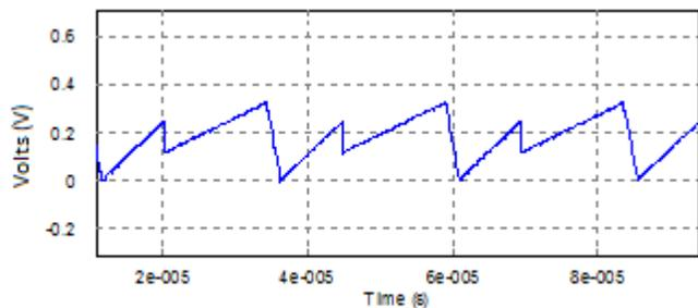
Figure 6. Sum of the sensed ramp and external compensation ramp ( $S_n+S_e$ ).
