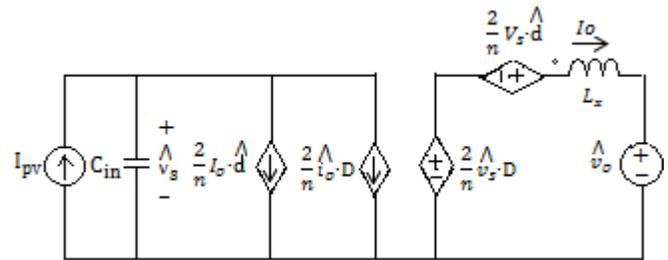
Figure 2. Small signal model of the push-pull converter.
