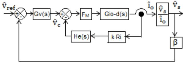
Figure 3. Control loops of current and voltage for the Push-Pull converter.
