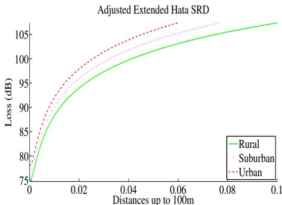
Figure 2. Path loss in three scenarios.
