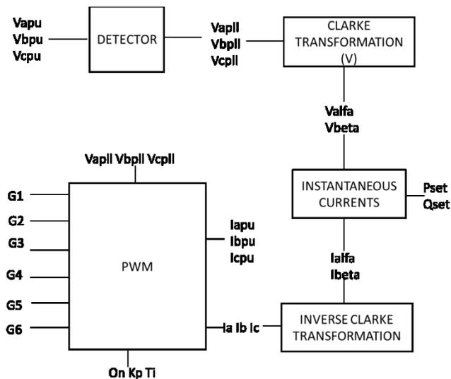
Fig. 4 P-Q based control scheme of the VSI
