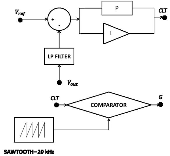
Fig. 2 Control strategy for the DC/DC Converter
