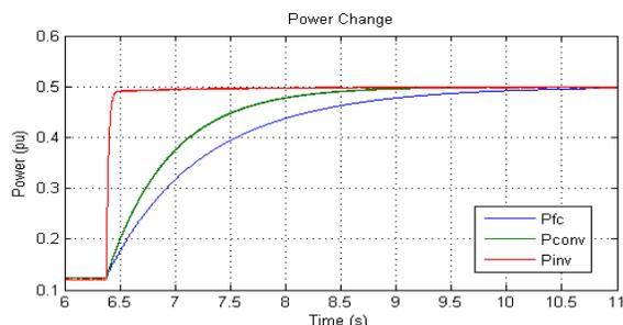
Fig. 7 Power Characteristics for a step change
