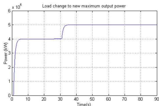
Fig.9 SOFC generating 500 Kw
