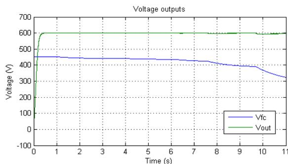
Fig. 6 Fuel cell voltage and converter output voltage
