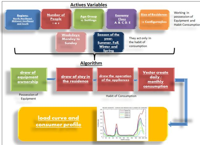
Figure 1. Schematic of Algorithm for Load Curves Construction.
