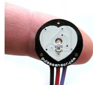
Figure 3: We used a pulse sensor (made by pulsesensor.com) and connected it to the Raspberry Pi. With software from this website students were able to obtain their pulse readings and record it automatically into a database.
