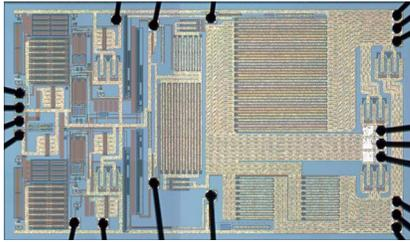
Fig. 3. Chip micrograph of the designed pulser.
