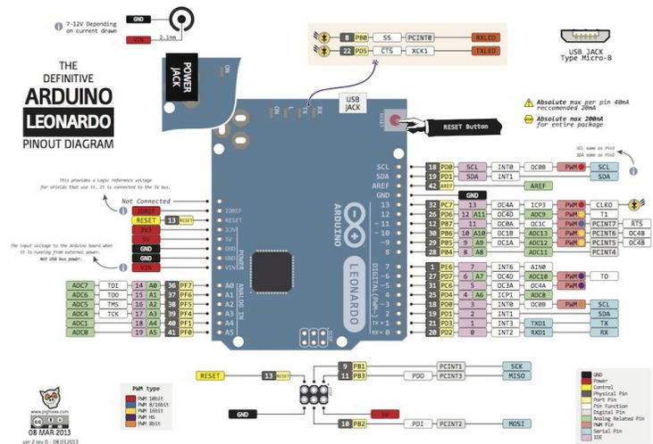
Fig. 1 Arduino leonardo microcontroller module pin
