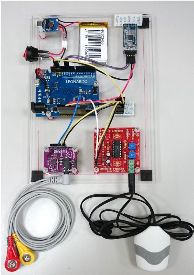
Fig. 2 ECG & PPG signal acquisition device
